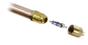
The 36LP Series comes with a CD2250 wrench cap and CD4460 valve core and is available in a variety of tube sizes ranging from 1/8" to 3/8". There are no pipe threads. Material is CDA 360 brass and standard refrigeration tubing. Tube length is approximately 2".
