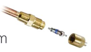
The T 36 Series comes with a CD2250 wrench cap, CD4460 valve core and is available in a variety of tube sizes. There are 1/8" male pipe threads below the hex. Material is CDA 360 brass and standard refrigeration tubing.
